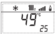
24. Visualisation safety thermostat with board ZONA MIX 2 (input S1) respectively ON and OFF
